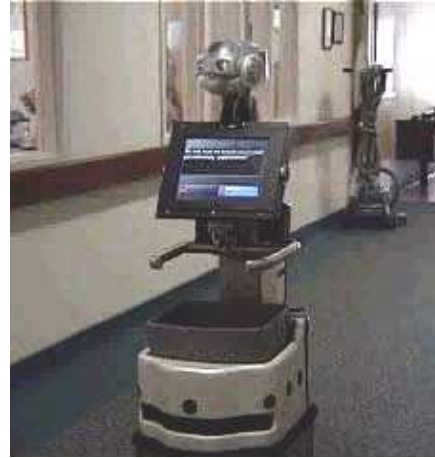
Figure 1: Pearl, the CMU Nursebot (courtesy, Carnegie Mellon Robotics Institute), is able to remind elders of their activities and lead them to the activity if necessary
