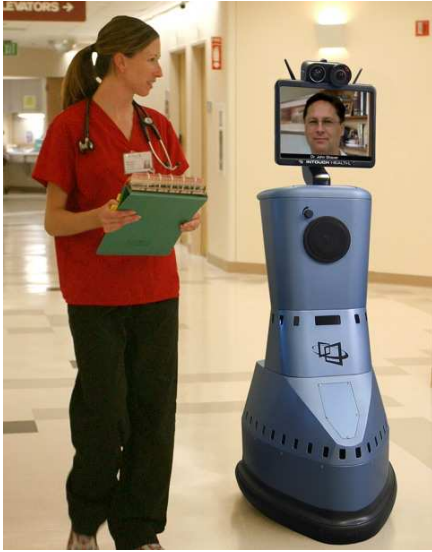
Figure 2: The InTouch RP-7 has been in long-term care facilities such as the Silverado Senior Living Aspen Park facility since 2003. There it is used for remote visits by high-level administrators and staff training mentors, or by corporate nurse consultants for patient examinations (Winner 2007)
