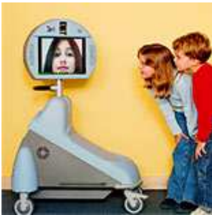
Figure 3: Pebbles is a mobile teleconferencing application that attends school for disabled children—allowing them to maintain relationships with their peers. Pebbles includes a rudimentary manipulator for interacting with the teacher in a classroom setting.
