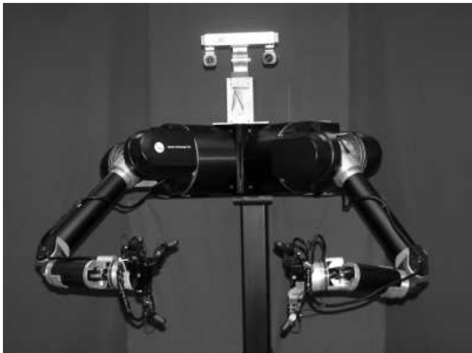
Figure C.1. Dexter, the UMass bimanual humanoid.
