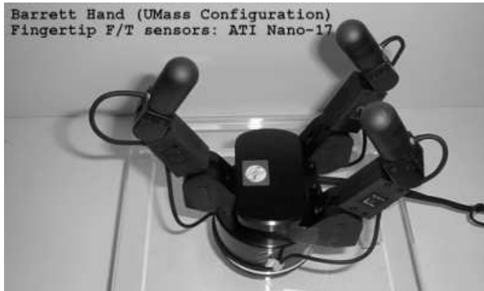
Figure C.2. Dexter’s two Barrett hands are equipped with fingertip load cells.
