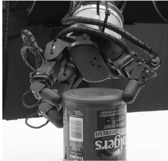
Figure 4.2. A grasp that uses a virtual contact. The two contacts on the left constitute a virtual contact that opposes the physical contact on the right.
