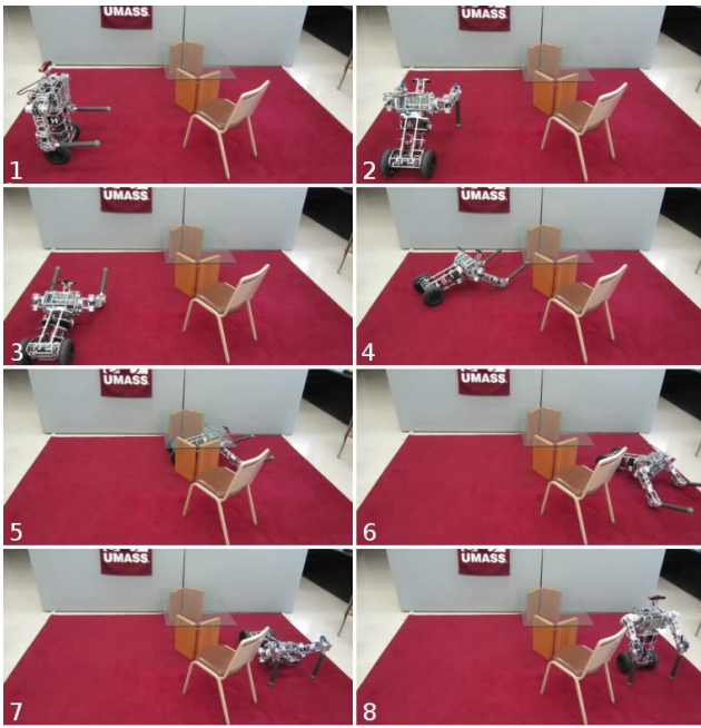
Fig. 10. Demonstration of prone scooting. uBot-6 is able to enter areas of the environment unreachable with balancing mobility. Here a chair and table block the path. After a transition to prone scooting the robot can pass under the table and stand up on the other side.
