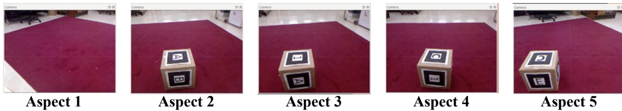
Fig. 4. ORBIT-Z re-orient the robot by moving it clockwise around the box. The effect of taking the ORBIT-Z action on this box is that the ARTag feature “4” becomes visible.
