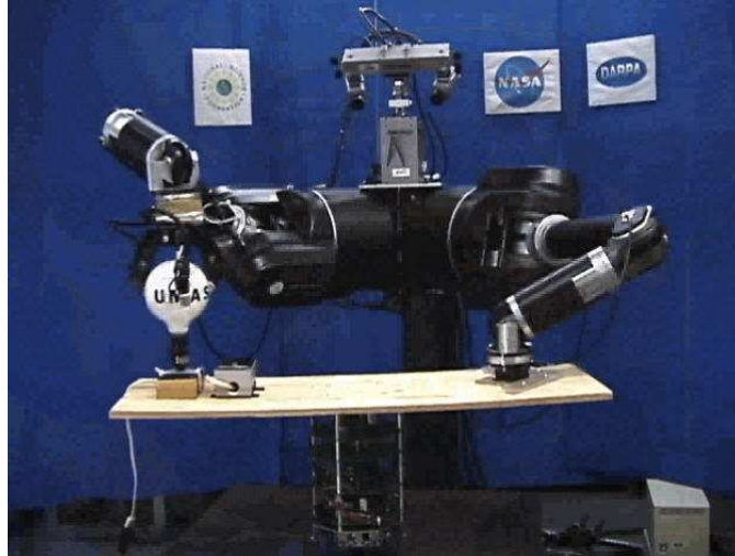
Figure 3.4. The uBot-2 presents dynamically stable environment to the Barrett WAM stationary manipulator in the task of screwing in a light bulb.
