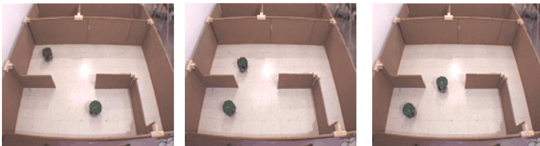
Figure 3.2. Two uBot-1 robots performing a maze exploration while maintaining the line-of-sight constraint.
