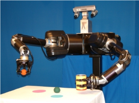
Fig. 2. The experimental Dexter platform for studying learning algorithms and control frameworks in bimanual dexterous manipulation.
